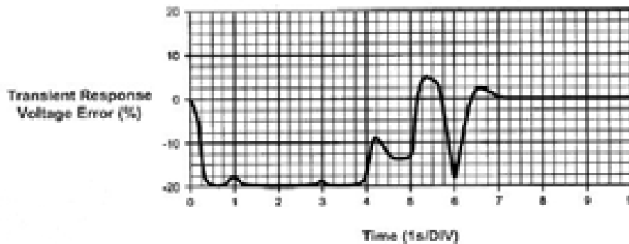
100% Diesel 100% Block Load
